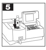
**5**. Zero the instrument using the zero vial (white cap) provided and read the sample.
